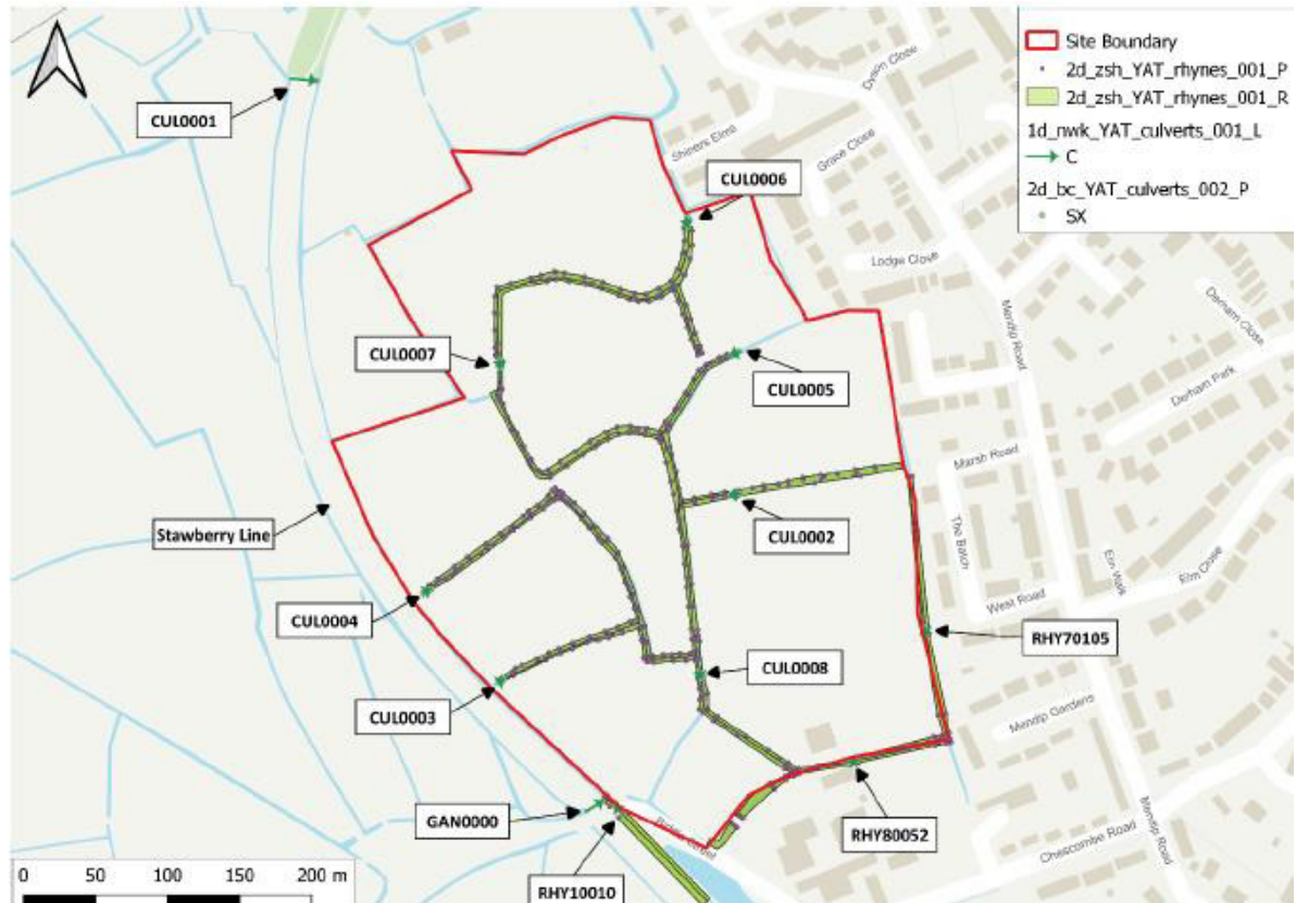
Figure 1-2 – Details of Rhyne Network adding to model to better represent site drainage conditions.
