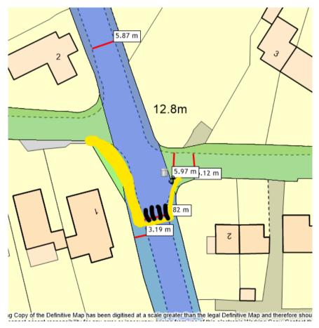
The footway width as shown in the image below is substandard and we **require** the developer to make improvements at this junction to widen the footway to a minimum of 1.8 meters to match Brinsea Road. Improvements to be delivered by Section 278 agreement (as within the adopted highway) and secured by **condition**.
