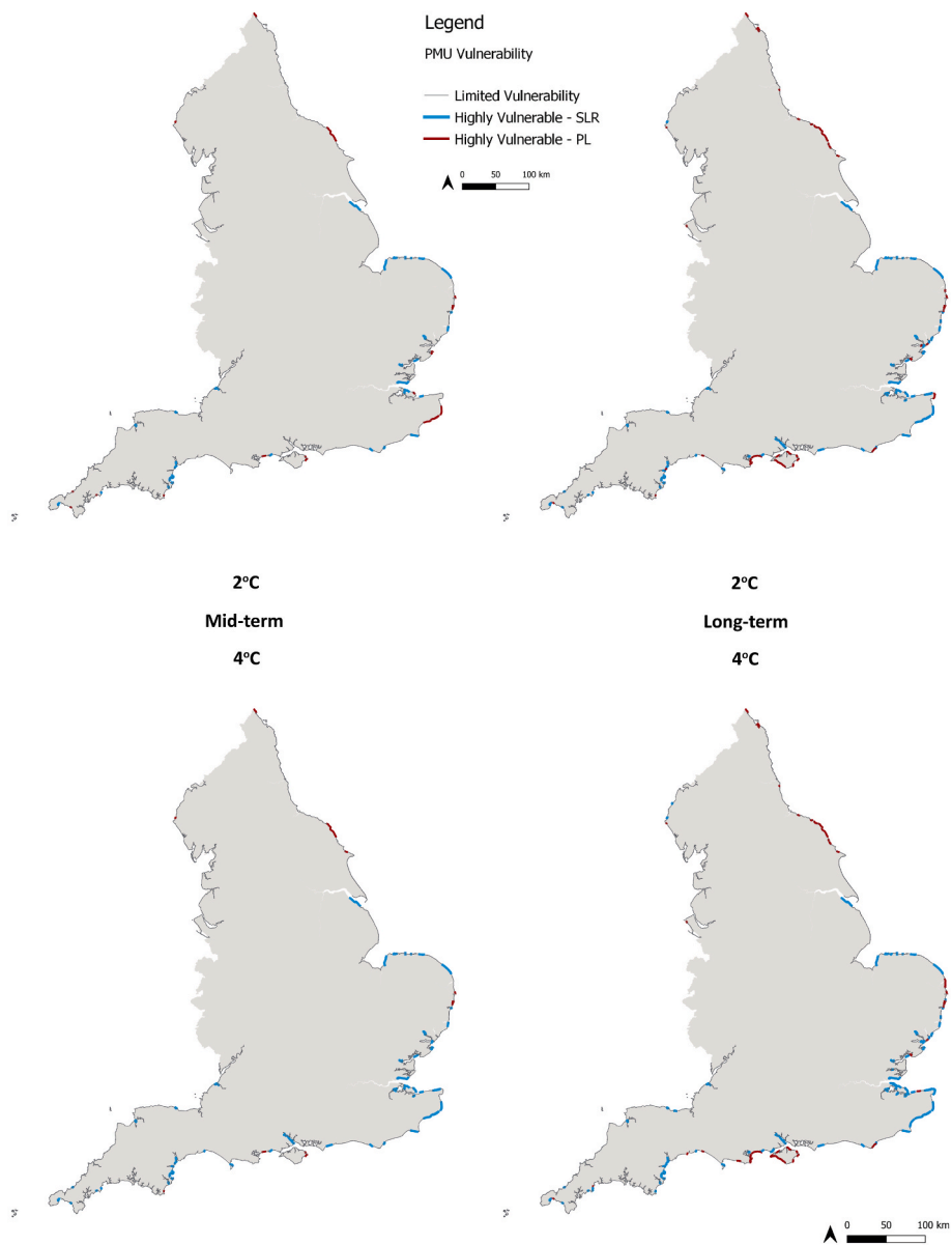
Fig. 11. Coastal (flood) defences vulnerable to either sea level rise or wave-driven shore platform lowering. Top: 2 °C rise in GMST – relative SLR and platform lowering. Medium and Long term. Bottom: 4 °C rise in GMST – relative SLR and platform lowering. Medium and Long term.
