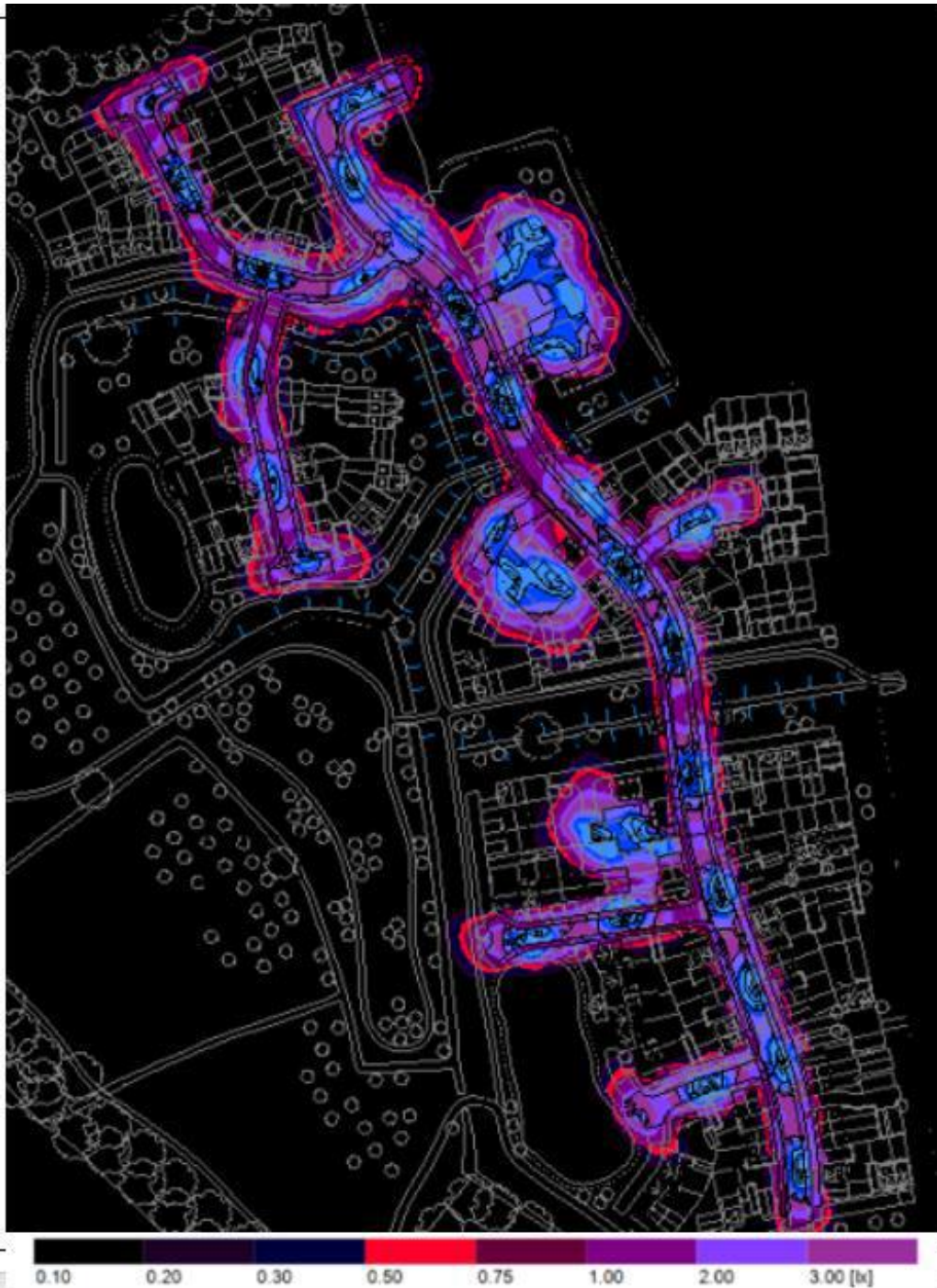
Figure 5: External Lighting (lux contour plan) from Lighting Assessment Report by e3 consulting engineers, document reference: 4790 REP01 based on the illustrative masterplan.
