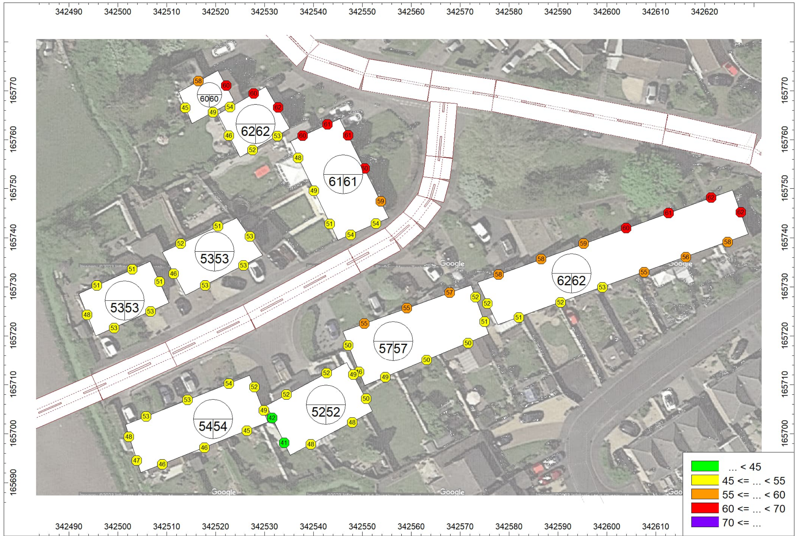
Figure 4 Committed + Proposed Development year of opening 2025 (Do Something) modelled noise levels based on AAWT figures (Shiners Elms link 1)
