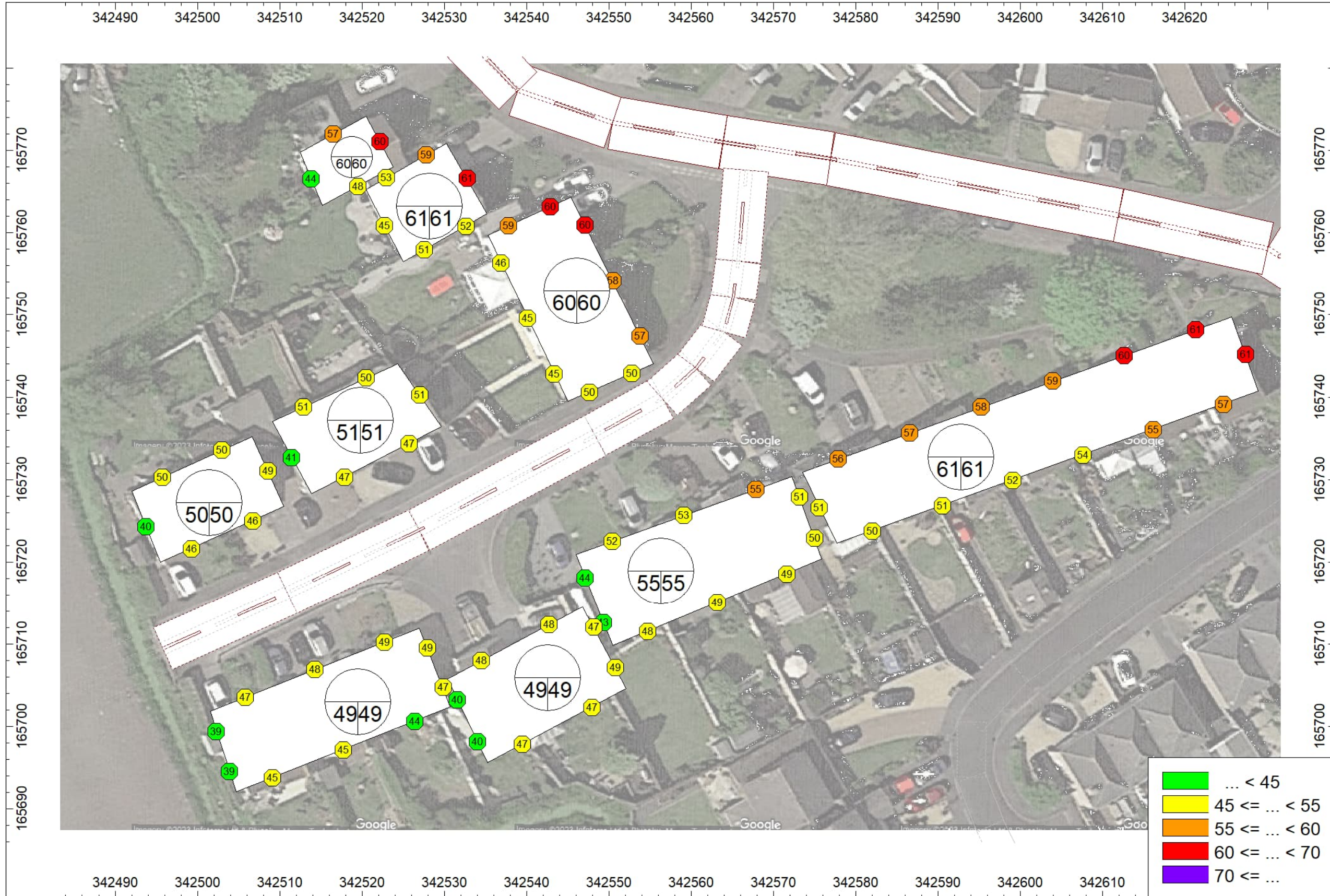
Figure 3 Committed Development year of opening 2025 (Do minimum) modelled daytime noise levels based on AAWT figures (Shiners Elms link 1)
