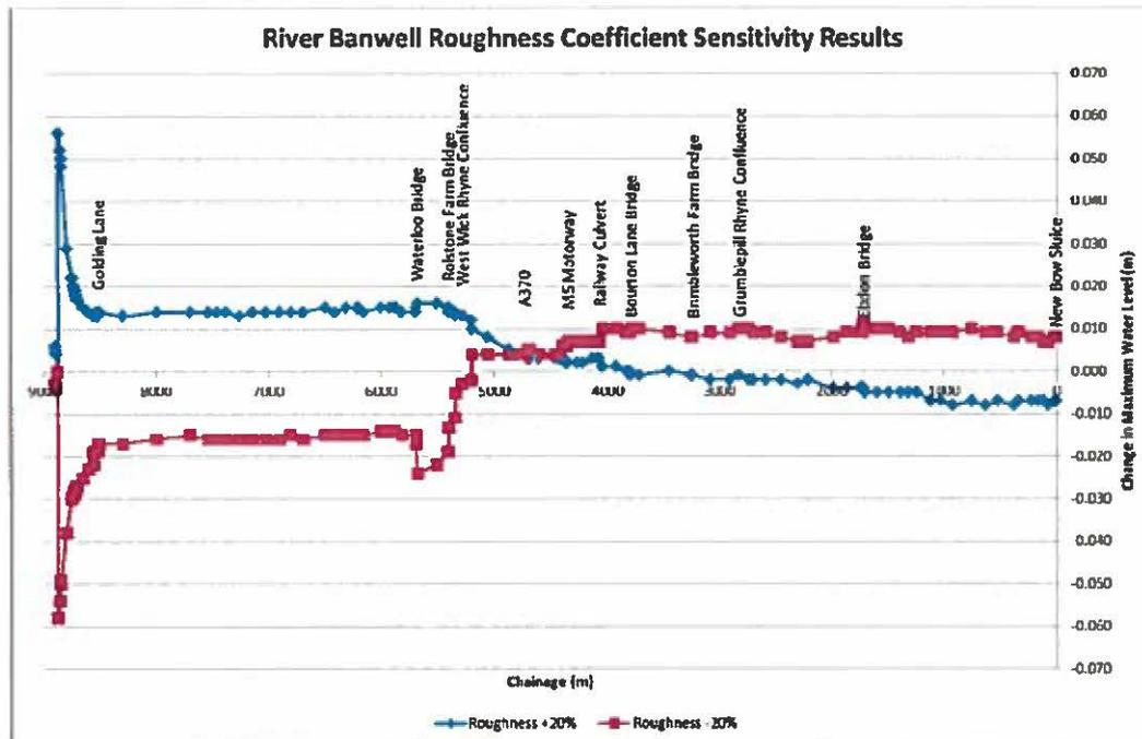
Figure 8.4: River Banwell Changes in Peak Water Level due to Change in Roughness Coefficient
