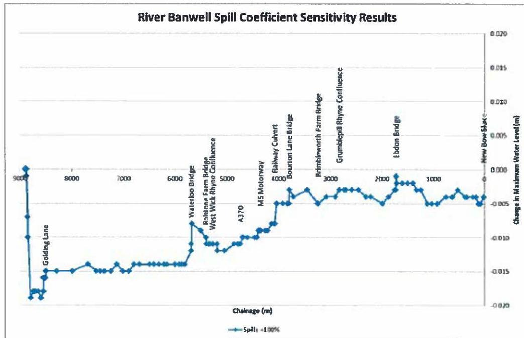
Figure 8.5: River Banwell Changes in Peak Water Level due to Change in Spill Coefficient
