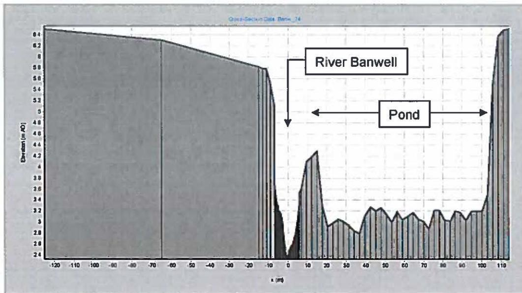
Figure 6.5: River Banwell Additional Storage Feature Typical Cross Section
