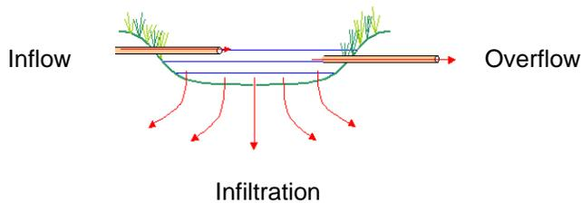
Figure G1d - Cross-section of a Pond
