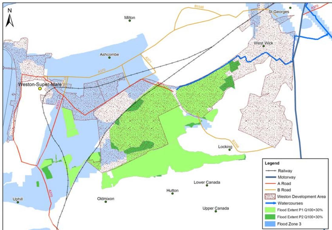
2.3.8 Within the Banwell catchment there is not a significant increase in flood extents between pre and post development. Figure 2.6 shows the current Flood Zone 3 (1% probability) extents for the Banwell catchment compared with the extents of the 100 year return period flows plus 30% for pre and post development derived from the hydraulic modelling. More detail of the flood extents is provided in drawing AA\_0103 in Appendix A.
