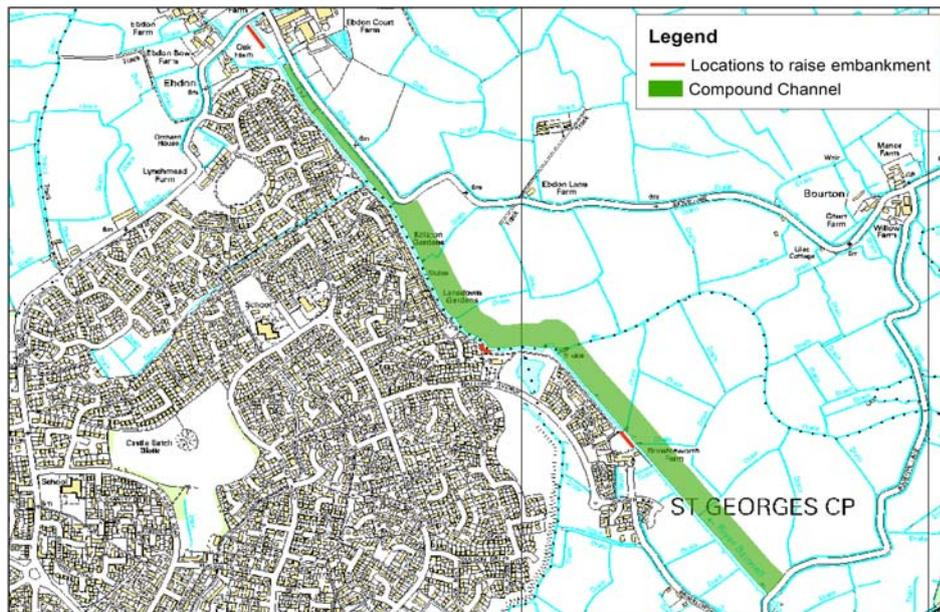
A compound channel would be constructed downstream of the M5 motorway with a lowered bank extending laterally for 50m on the right bank of the channel over a 1900m stretch of channel. This will provide additional storage and lower water levels locally at times of high flow with minimal disruption to the existing agricultural land use (grazing). At certain points along the left bank of this channel the defence is known to have low points which would require a small increase in elevation.
