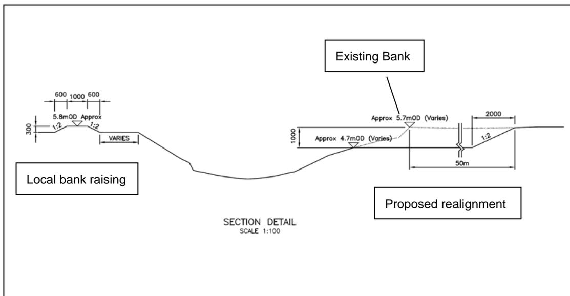
5.3.4 There are three locations where the channel is known to have low points requiring the existing embankments to be raised by up to 300mm to ensure that the freeboard is not compromised. Material for this work could be brought in from the compound channel excavations if suitable. The length of bank to be raised totals 190m and the locations are identified on figure 5.7.
