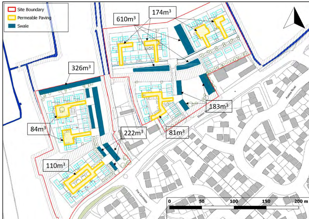
Figure 8: Location of Permeable Paving and Swales
