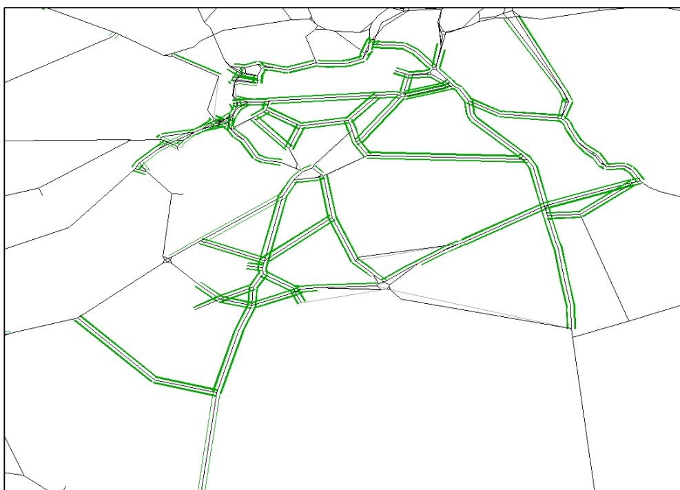
Figure 3.3: SATURN network of links which have been converted from fixed to variable speed
