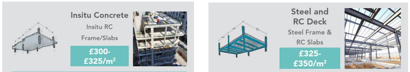
Figure 3-10 – Typical frame construction cost for insitu concrete frame and slabs (left) and steel frame with reinforced concrete slabs (right)
