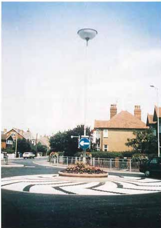
Mini-roundabouts and changes in camber can cause a bus to lean, endangering standing passengers. (Courtesy: Reading Transport Ltd).
