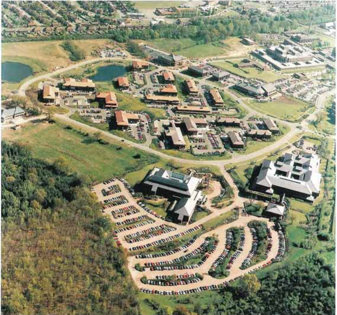
Guildford science park with the Royal Surrey Hospital in the background. Note the extensive car parking, the only possible bus route and the poor pedestrian access from the bus route to some buildings. (Courtesy: Aerofilms Ltd).
