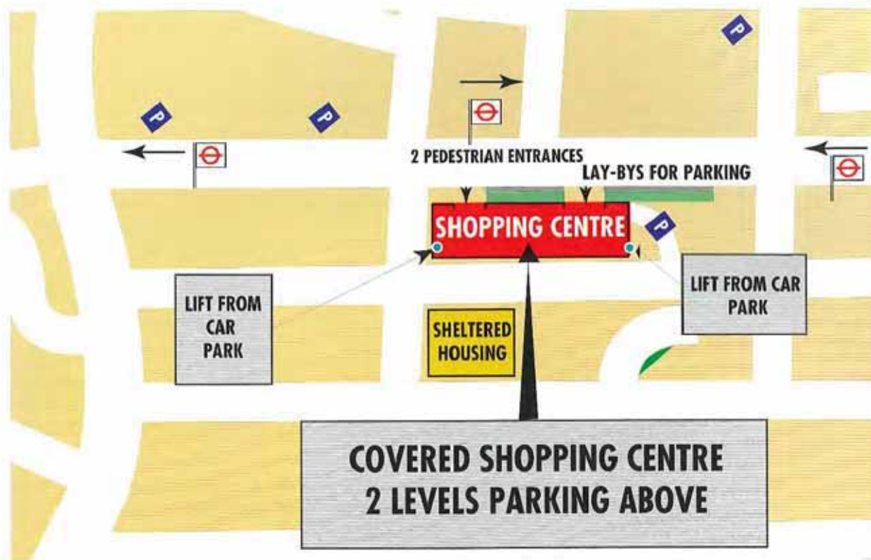
Fig 6.2: A shopping centre with better access by car than bus.
