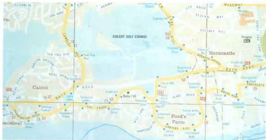
Fig 6.3: A well designed housing development with a central spine bus route and bus gates to stop car traffic. (Courtesy: Reading Transport Ltd).
