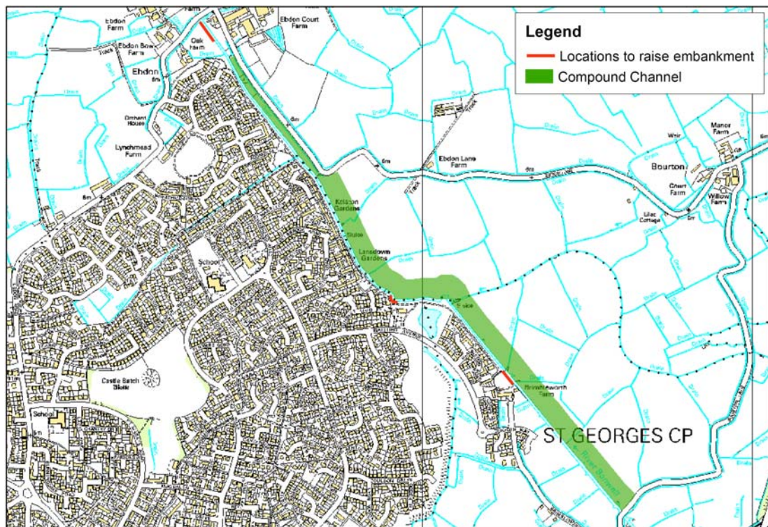
Figure 5.7 Banwell catchment: Location of compound channel and raised embankment work
